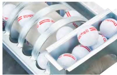
The rotating brush moves the balls through the spiral.
